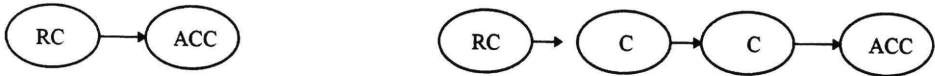
Figure 1 Single Root-Cause Model with one antecedent causing the accident (left) and Extended Root-Cause Model in which the immediate cause of the accident is derived to an earlier root-cause (right). RC = root cause, C = cause, ACC = accident.
